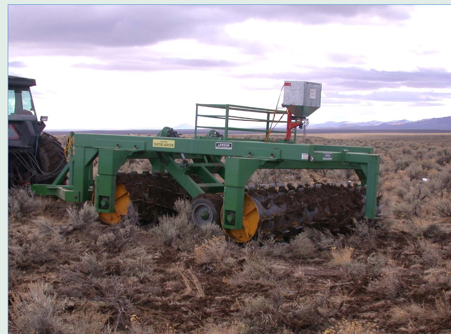
Figure 1. Lawson Aerator purchased by the USDA-ARS, notice the size, heaviness and steel plate teeth to crush old and decadent shrubs.
